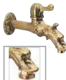
A696 Rubinetto curvo da giardino in ottone giallo trattato, 1/2 a leva, con rosetta pesante aeratore e riduzione 3/4 per portagomma. Plain-end garden bibcock, heavy duty in treated yellow brass, 1/2 lever type, with heavy flange, aerator and 3/4 reduction for hose connection.
