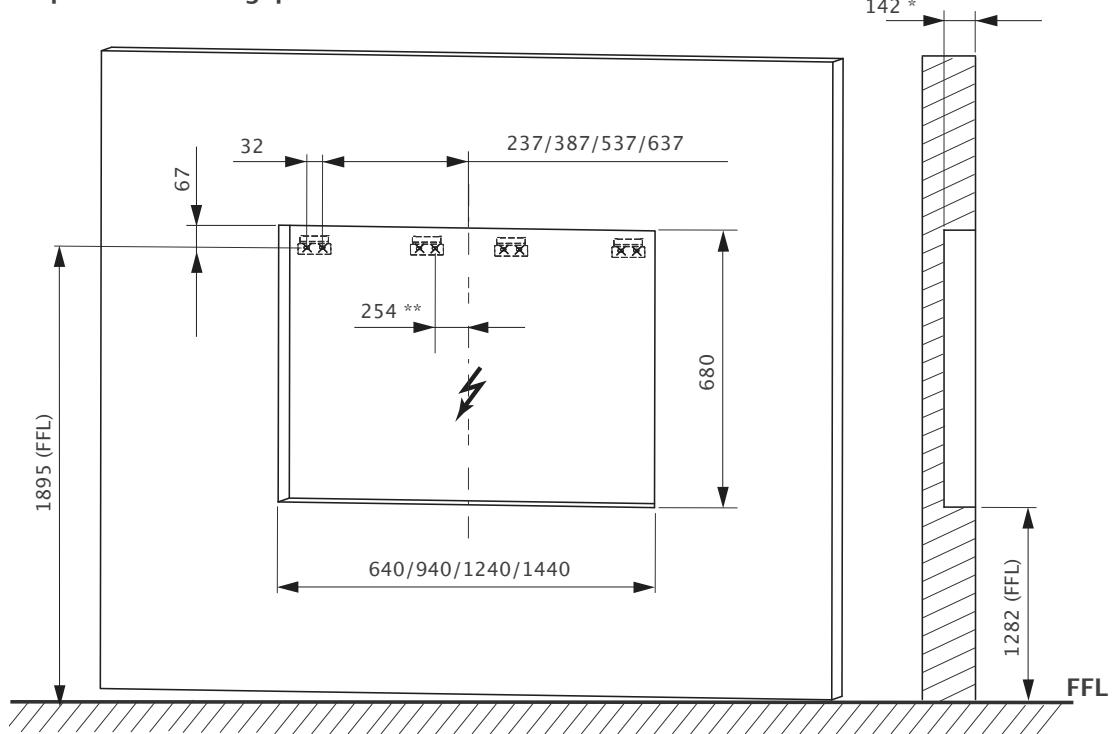
x = drilled position in the wall
