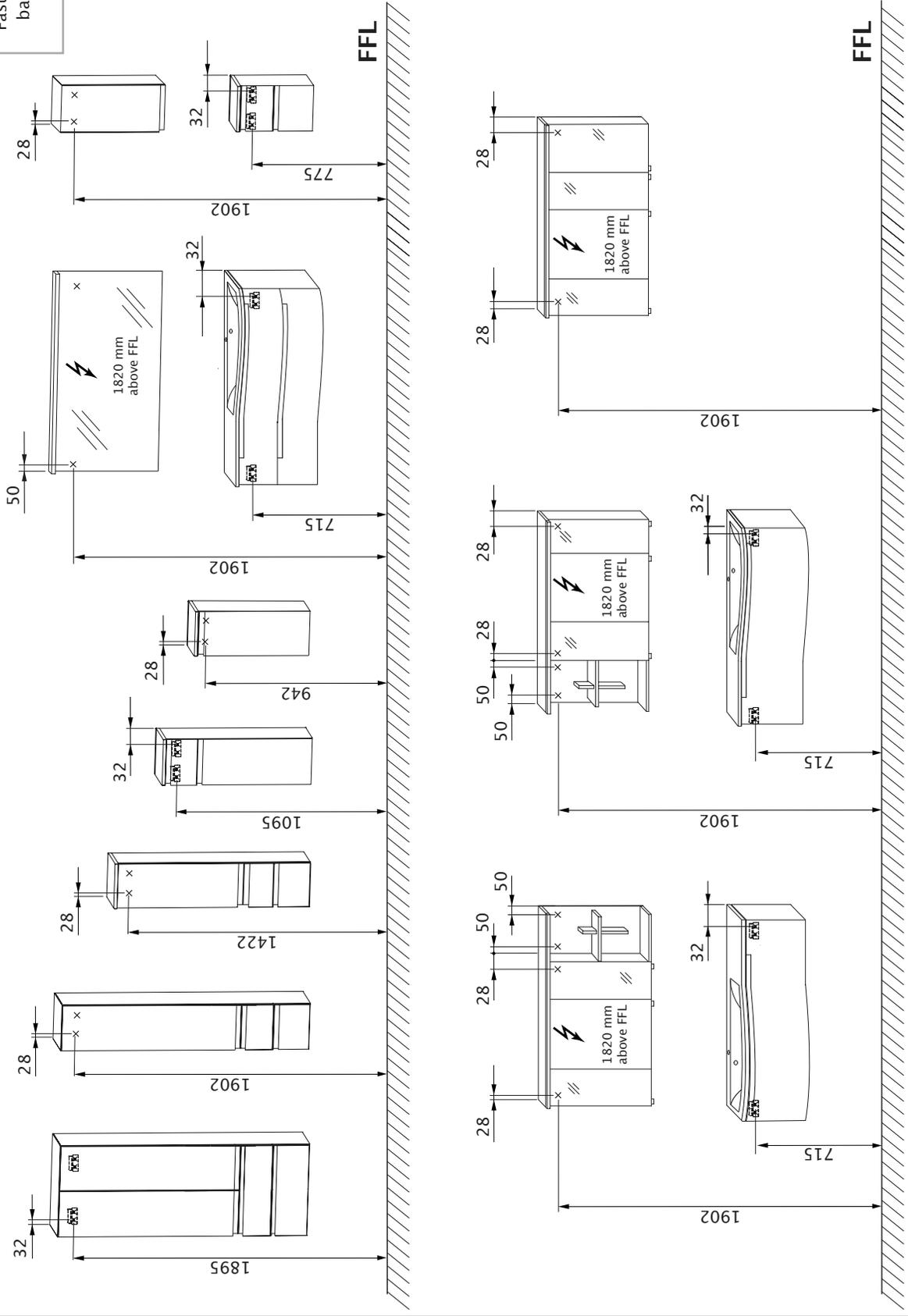
FFL = finished floor level      = Fastening on a strip      x = Fastening on a screw hook      x = drilled position in the wall
