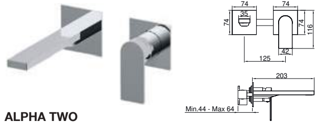
ALPHA TWO 01ALC180CR 11,7 l/min 3 bar
